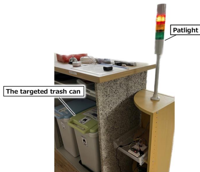
Figure 2. View of the colored light indicating saturation of the trash can
