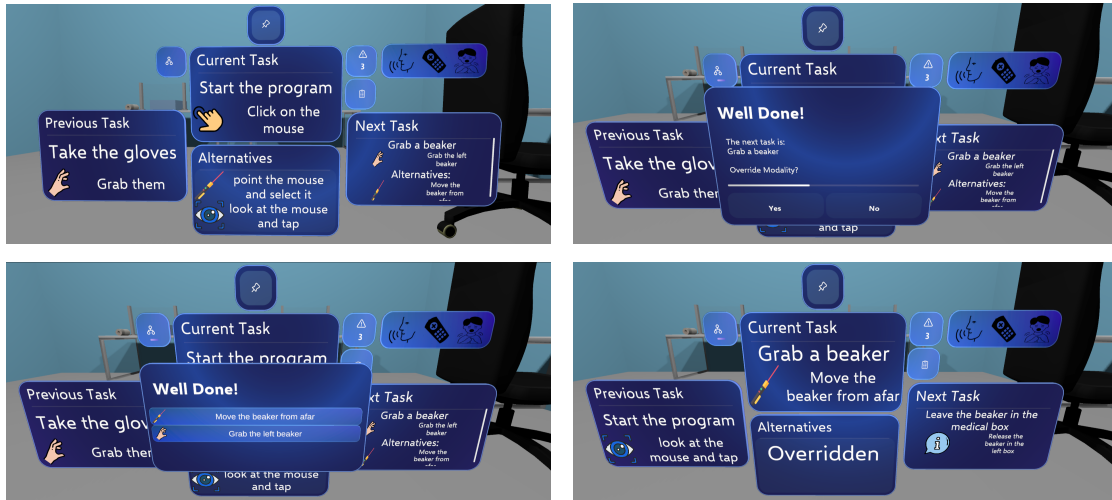
Figure 1: The current prototype interface. From top left to bottom right: The base interface, in its expanded version; the feedforward prompt; the modality choice list; the interface after a modality override.
