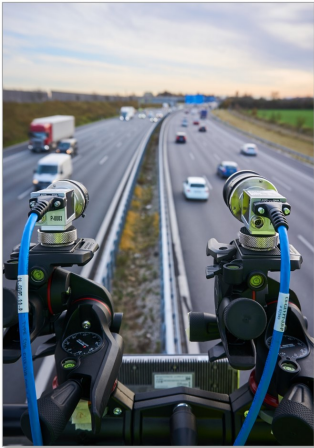
Figure 2: Picture of radars on the highway tracking the traffic.
