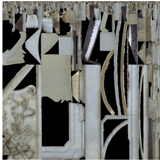
Figure 2: Color map of a sample segment. RGB information is computed by comparing high and low poly meshes.
