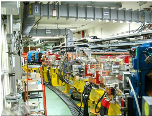
Fig. 6: Injection region of Delay Loop with the waveguides feeding the 1.5 GHz RF deflectors
