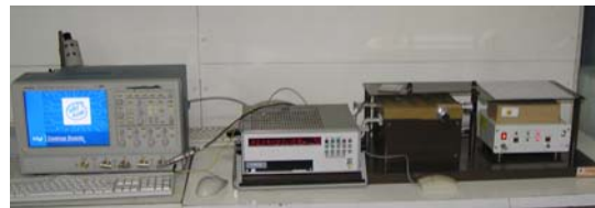
Figure 22. The MW-PCD measurement setup at the University of Vilnius.
