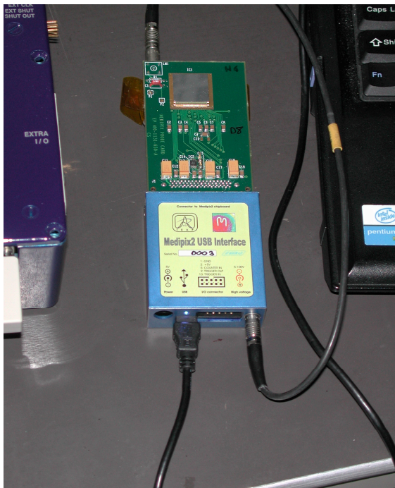
Fig. 1 Photograph of a complete module with sensor board and USB readout box in the middle. The USB cable at lower left connects to the portable computer at the right. The high voltage for the Si sensor, usually 100V, is provided from the USB module below to the top of the sensor board via the other cable with LEMO™ connectors. The undivided rear side of the 14 \times 14\text{mm}^2 sensor is facing you, while the matrix of contacts and the Medipix2 readout chip are behind the sensor. The assembly is glued on the green printed circuit board which also contains decoupling, of which 4 large capacitors are seen. A 120 contact, flat connector in the USB box holds this circuit in place, and provides communication between the USB circuits and the Medipix2 chip. All control signals and data are transmitted back and forth to the computer via the standard USB cable. To the left one can just see a small corner of the earlier serial readout system MUROS, which illustrates the progressive reduction in size of the readout electronics.
