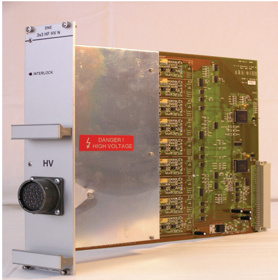
Figure 8: The high voltage supply module is shown above and it is housed in the HV crate (see Figure 6). The high voltage output is through the connector shown on the panel.
