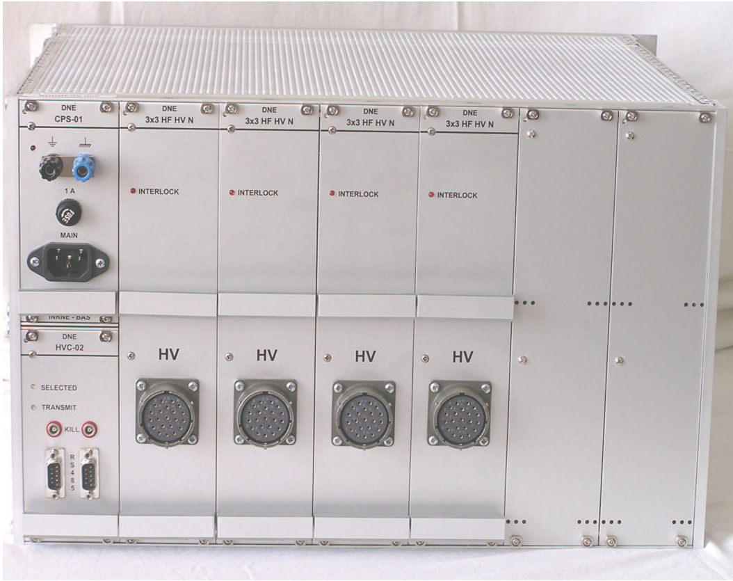
Figure 6: The high voltage crate normally houses 4 power supply modules, one per HF quadrant.
