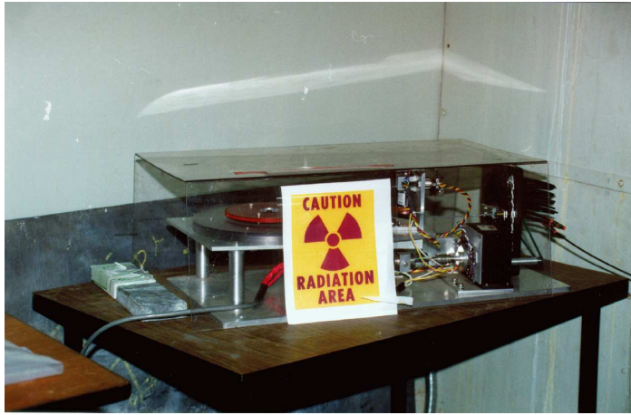
Figure 16: The driver of the radioactive source tubes which is used to test the HO trays
