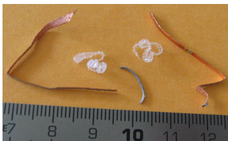
Figure 5: Some of the obstacles found in magnets in the tunnel.
