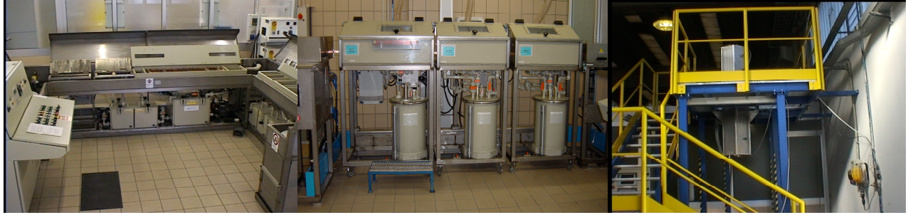
Fig. 6. Pilot plant for Bi-2212 : a) copper electrowinning ; b) Bi, Sr, Ca electrodeposition cells, c) furnace.
