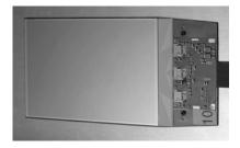
Figure 7. An IT module with one silicon sensor. The silicon sensor is  $7.8 \times 11 \text{ cm}^2$  in size. The three Beetle front-end chips are glued to the kapton hybrid and wire bonded to an Alumina pitch adapter.
