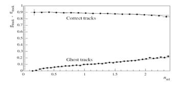
Figure 9. The tracking efficiency and the ghost rate for long tracks as a function of the relative hit multiplicity, i.e. the hit multiplicity of the tracking detectors divided by the average hit multiplicity.
