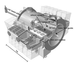
Figure 2. Schematic view of the Velo detector. The corrugated foil separates the beam and detector vacuum, and serves as an RF shield for the detector modules.
