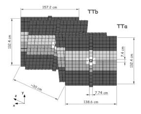
Figure 3. A schematic layout of the Trigger Tracker. The square elements represent the silicon sensors, which have a size of 9.44×9.64 cm<sup>2</sup>.
