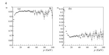
Figure 8. The tracking efficiency and ghost rate for long tracks.
