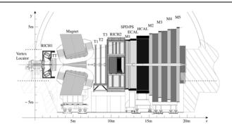
Figure 1. Schematic view of the LHCb detector.
