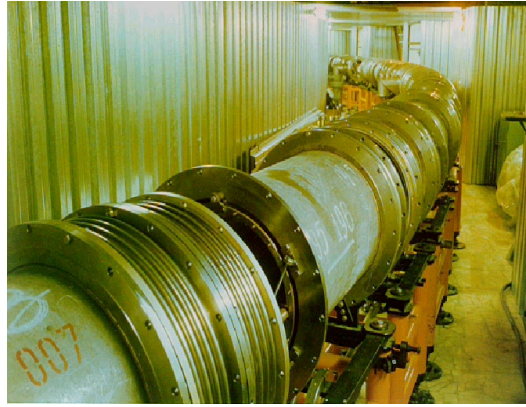
Fig. 2: The Nuclotron: a superconducting synchrotron for heavy ions up to 6 GeV/n. It has been operating since 1993.
