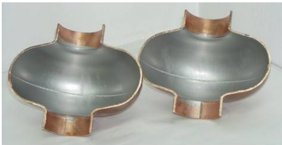
Figure JRA1.4.7: Two parts of the coated single-cell, which was cut in order to perform an analysis of the inner surfaces.
