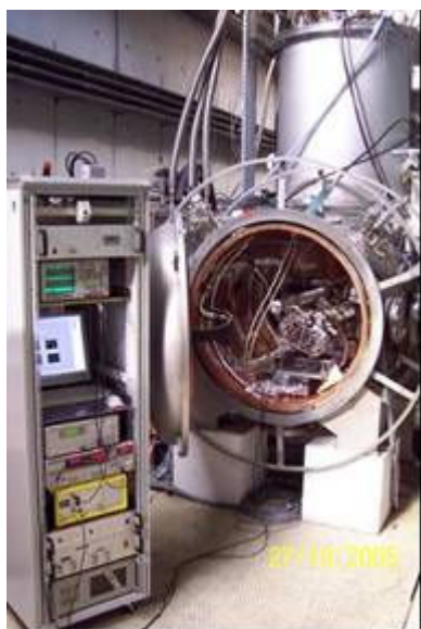
Figure JRA1.8.11: C45 TTF cavity in CRYHOLAB ready for integrated experiments. The electronics on the left allows characterization of mechanical modes of the cavity assembly: F, Q, piezo to piezo and piezo to frequency transfer functions.
