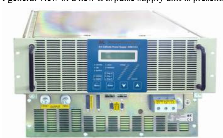
Figure JRA1.4.3: new DC/pulse power-supply for the linear-arc facility.
