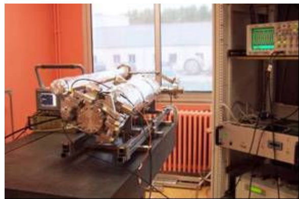
Figure JRA1.8.10: The piezo tuner is mounted on C45 TTF cavity with the electronics in the laboratory.
