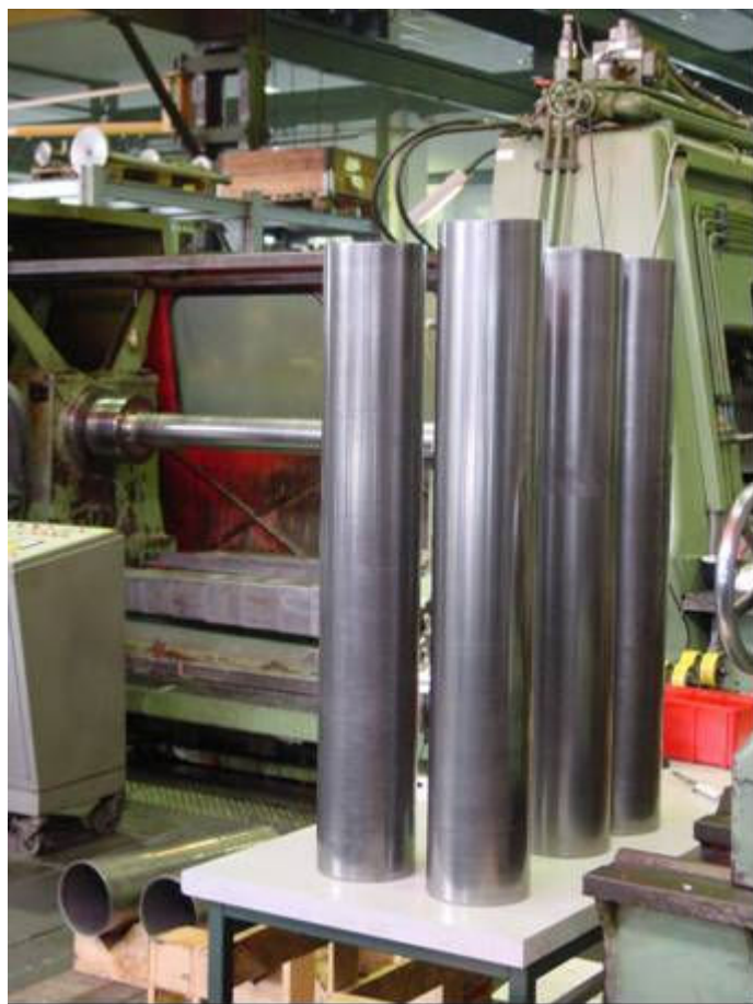
Figure JRA1.3.6 Seamless niobium tubes for cavity fabrication by hydroforming
