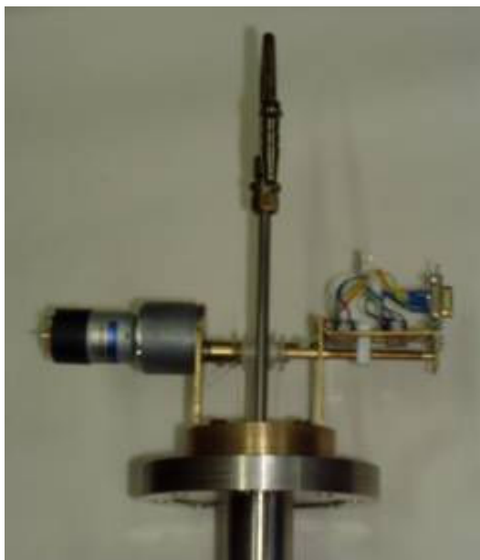
Figure JRA1.4.6: Top part of the magnet-drive system used in the modified UHV linear arc facility.
