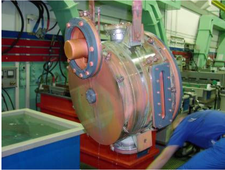
Figure JRA3.2.14: Copper-plating of CERN CCDTL pre-prototype.
