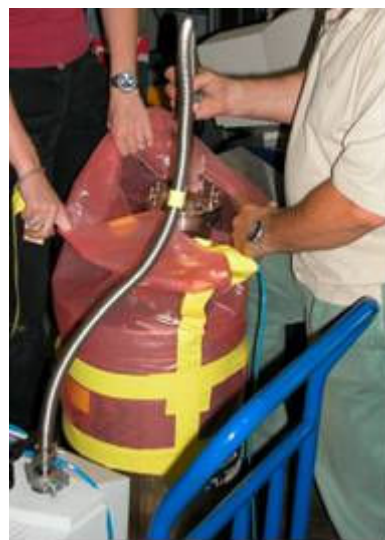
Figure JRA1.2.6: Bolt tightening with torque meter and liquid nitrogen temperature leak test.
