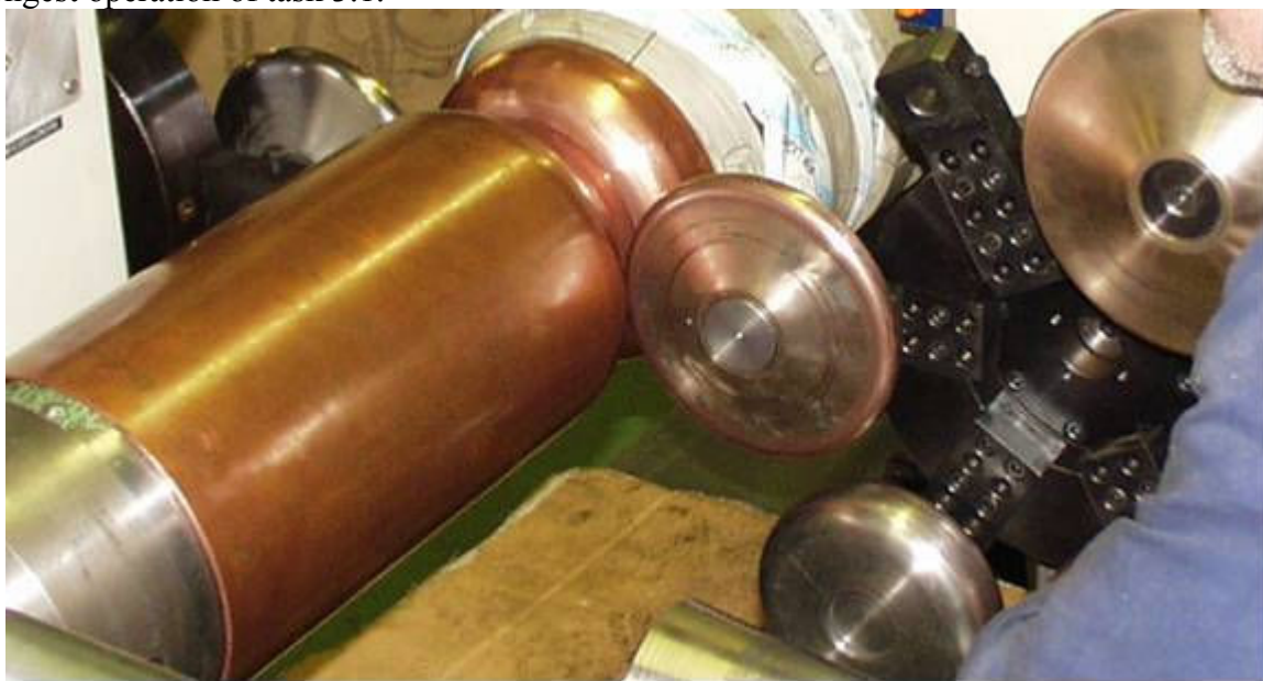
Figure JRA1.3.1: Phase of the double turret necking process during the spinning parameter definition action.
