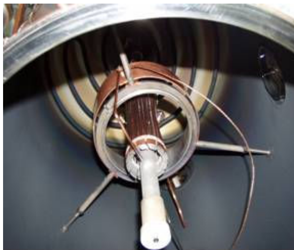
Figure JRA1.4.12: Picture of the cylindrical magnetic filter and an additional anode after the exploitation tests.
