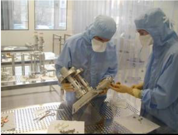
Figure JRA1.7.5: Coupler assembly in class 10 clean room.
