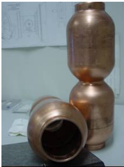
Figure JRA1.3.4: Necking at the tube end and tube middle implemented by necking machine.
