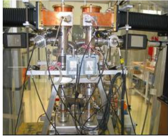
Figure JRA1.7.6: TTF-III couplers being conditioned.
