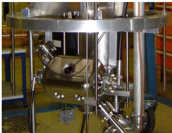
Figure JRA3.3.10: Niobium cavity mounted on the cryostat girder.
