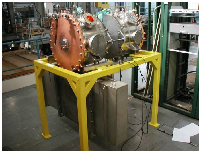
Figure JRA3.2.16: The assembled CCDTL pre-prototype. On the bottom can be seen the waveguide coupling port.
