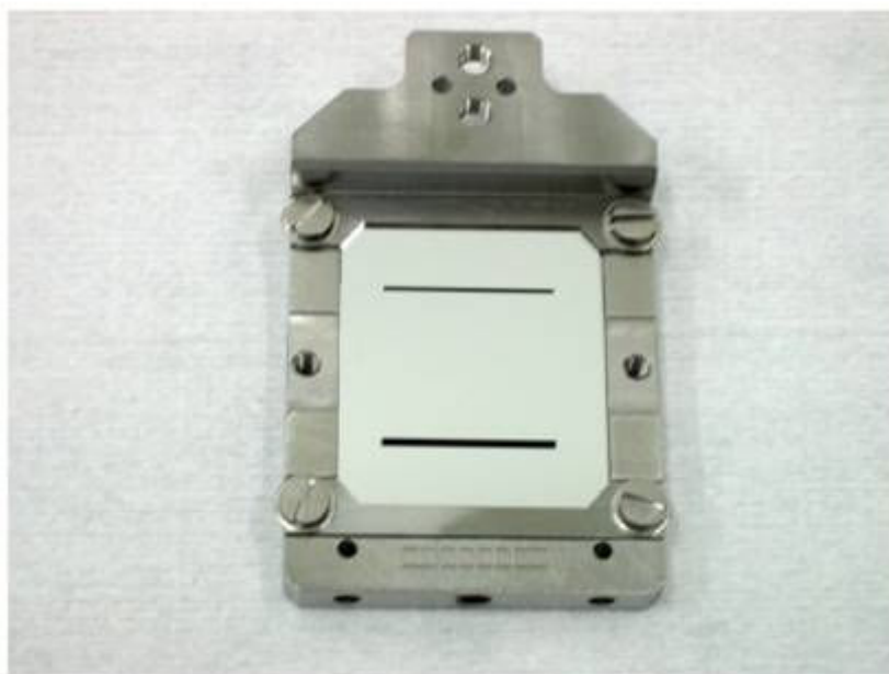
Figure JRA1.11.10: The DR screen with two slits of 0.5 and 1 mm respectively.
