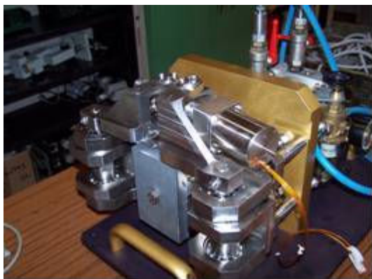
Figure JRA1.8.9: The measured stiffness on this test bench is 35 kN/mm limited by mechanical plays in ball bearing housings.
