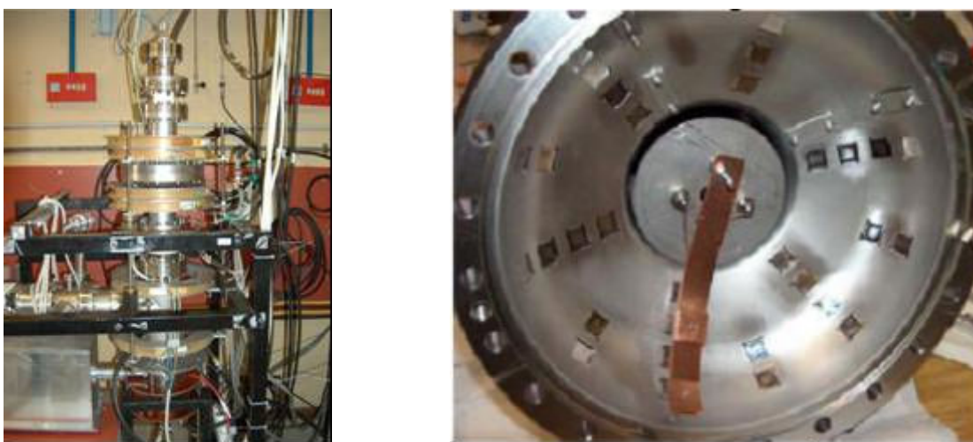
Figure JRA1.4.16: View of the unfiltered planar-arc facility for the single-cell deposition (left) and a picture of the inner surface of the upper half-cell with sample holders (right).
