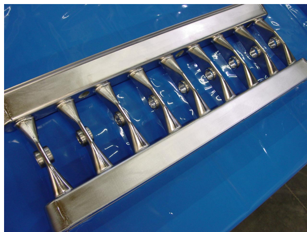
Fig. JRA3.3.5b: Welded Niobium girder + stem part of the sc CH-cavity for HIPPI
