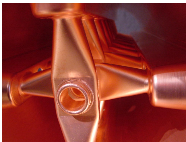
Fig. JRA3.3.5c: Niobium girder + stem part welded in the resonator of the sc CH-cavity
