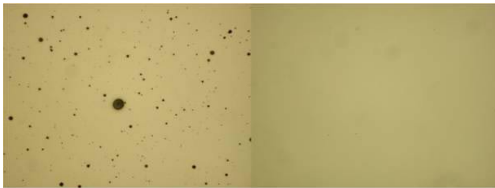
Fig.JRA1.4.13: Microscope pictures of the identical regions ( 250 \times 190 \mu\text{m}^2 ) of the sample coated without magnetic filter (left) and that produced with the active filter (right).
