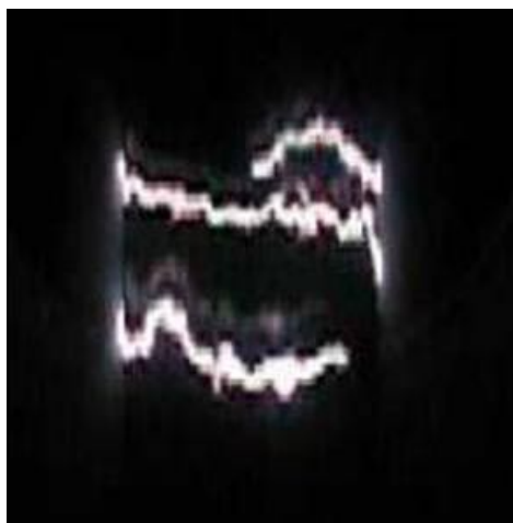
Fig.JRA1.4.7: Picture of the linear-arc discharge upon the cylindrical cathode surface, as observed at the base pressure of 4 \times 10^{-10} mTorr, arc current of 40 A, the action lasting 1 mn.
