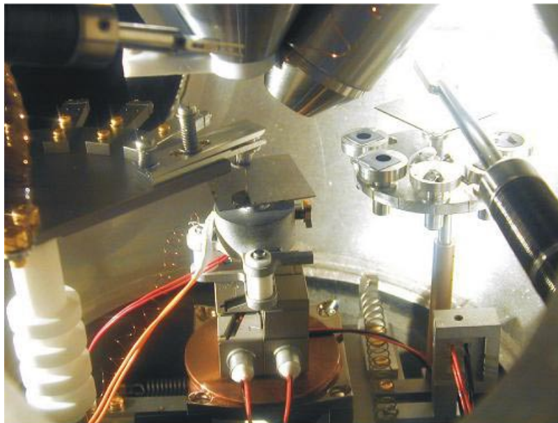
Fig.JRA1.6.5: View into the centre of the FESM: The sample holder can be seen in the middle of the picture. Above this table the fork system of the scanning needles (with different tip size) is installed.
