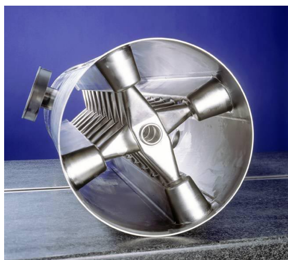
Fig. JRA3.3.5d: The superconducting Niobium CH-prototype cavity before the final welding of the end cells.
