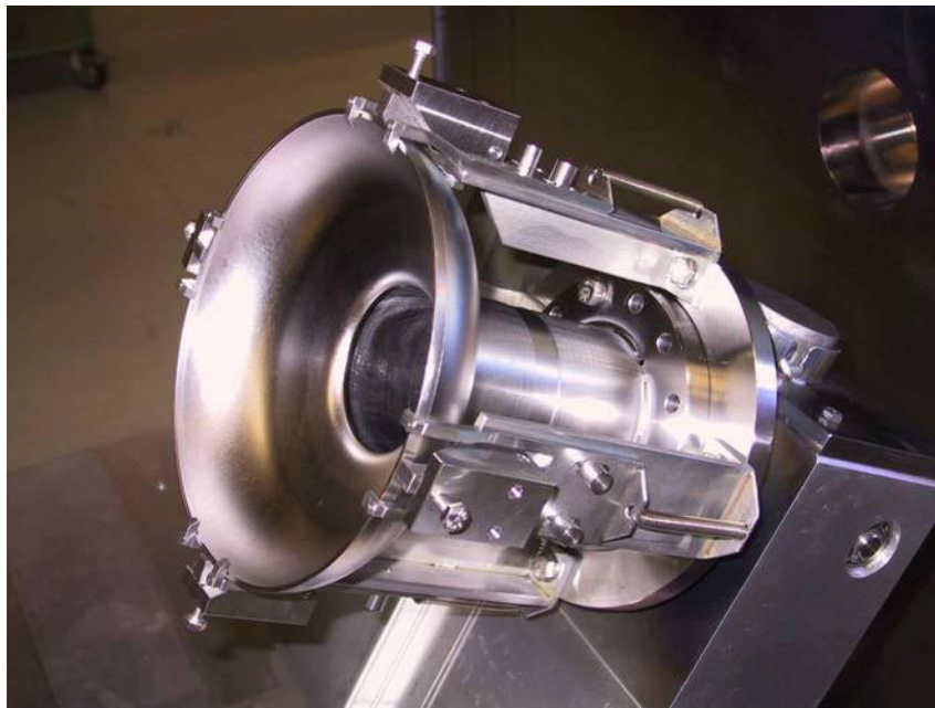
Fig.JRA1.2.12: Welding fixture for the iris seam
