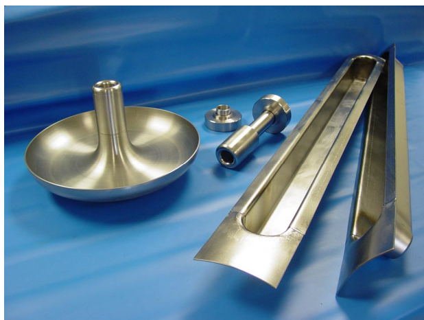
Fig. JRA3.3.5a: Some Niobium parts of a sc. CH-prototype for HIPPI. Tank end cell (left), two girders (right) and one drift tube part (middle)
