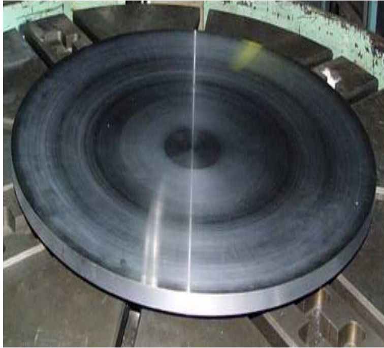
Figure 7: The beryllium blank (20 mm thick, \varnothing 800 mm) at Kompozit before machining.
