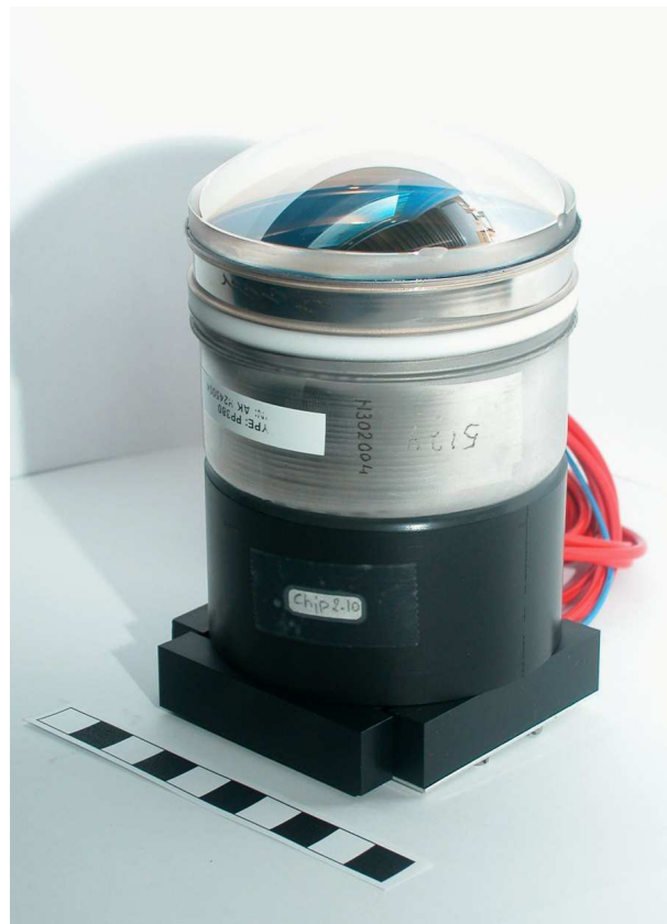
Figure 4: The pixel Hybrid Photon Detector.
