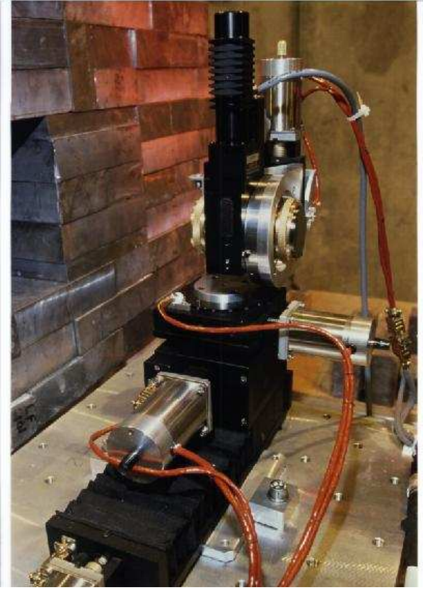
FIG. 11: Birefringent (quarter wave plate) Si crystal and goniometer.
