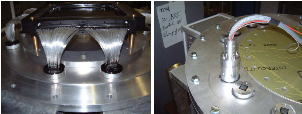
Fig. 5. The physical arrangement of the Sci-Fi tracker. The left hand figure shows one plane mounted inside the vessel. The black frame at the top encloses the scintillating fibres, and the clear routing fibre bundle can be seen. The right hand figure shows the front faces of the fibre bundles, with a PMT mounted onto one of them.
