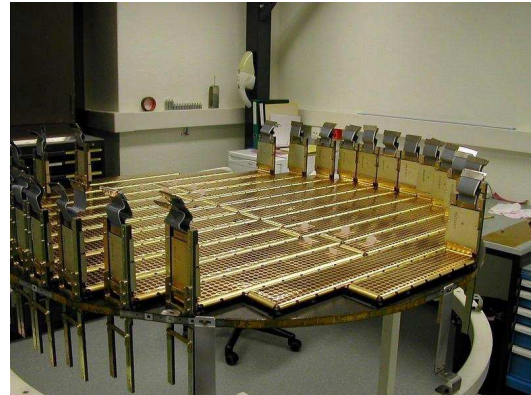
Figure 4. One of the inner plane equipped with ladders.
