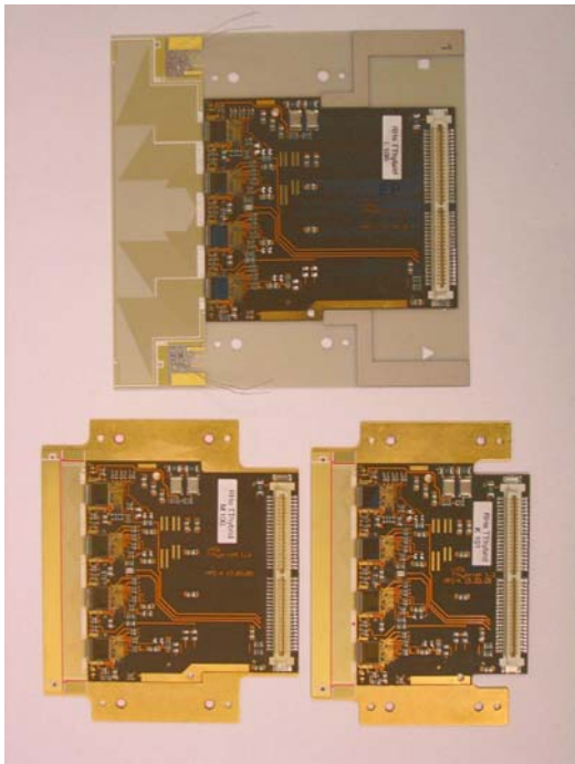
Figure 1: Photograph of the three hybrid subtypes for the TT detector. The hybrid at the top of the picture shows the lowest hybrid level.
