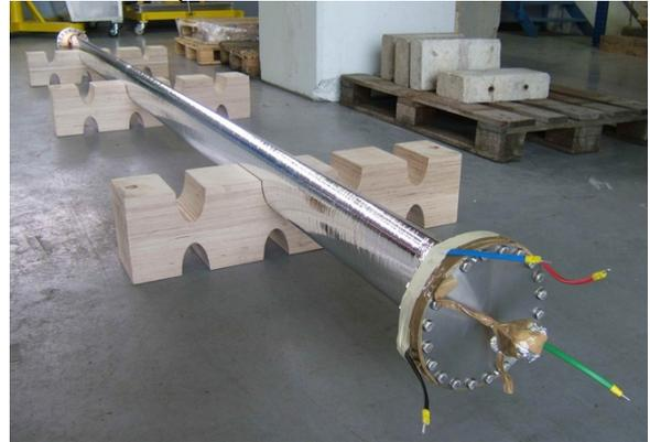
Figure 1: Finished MBXW chamber.
