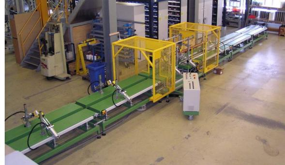
Figure 7: Wrapping machine; insertion table left, wrapping unit middle, traction unit right
