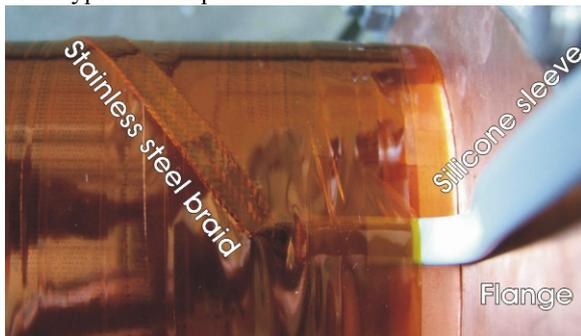
Figure 3: Electrical connection of heater bands.
