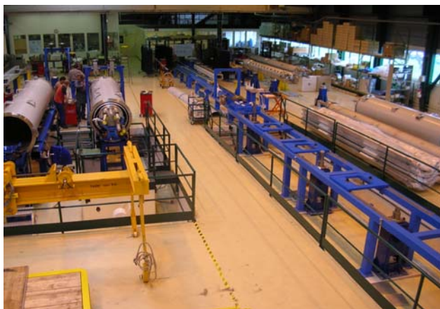
Figure 5: MS SSS Assembly benches: SSS with 2 supports (left), SSS with 3 supports (right).
