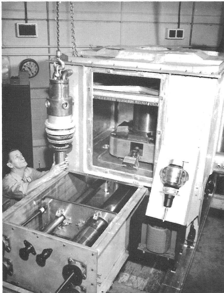
Fig. 2 ORIC power amplifier. The grid tank circuit extends forward from beneath the housing of the plate tank circuit. The RCA-6949, suspended at the left, fits inside the central conductor of the variable transmission line of the plate tank circuit. One of the four variable vacuum capacitors for fine tuning of the plate tank circuit is shown on the filament transformer at the right.
