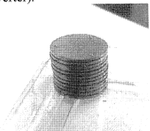
Figure 9: View of a piece of the target with 0.3 mm bumps. The target consists of 123 pellets (15 mm diam.) Each pellet is about 1 mm thick overall (0.7 mm + 0.3 mm).
