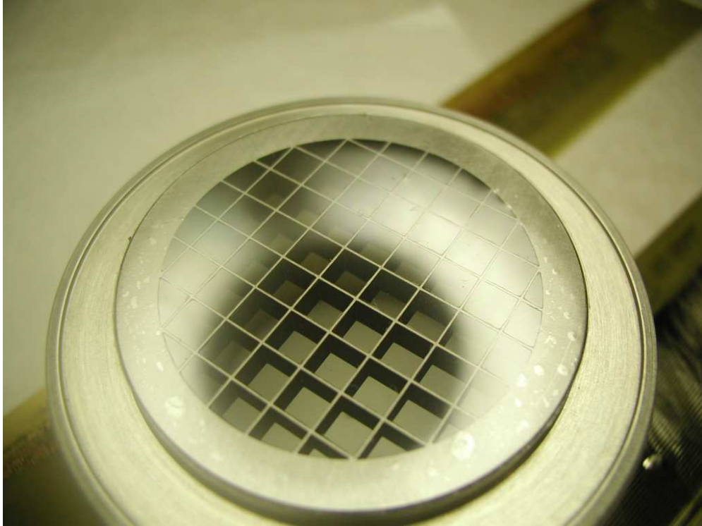
Figure 14: A sample cold window before the cryo and vacuum tests. The flange and the cell structure of the strong-back is visible. The window itself is glued from the back side to the strong-back.
