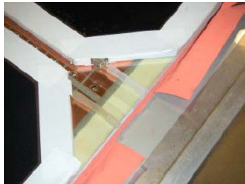
Fig. 9 Gas inlets of the top gas gaps, the readout strip and ground copper sheet can be seen below.
