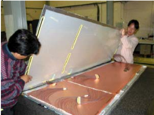
Fig. 10 Ready for top cover the after closing the Faraday cage with top Copper sheet.
