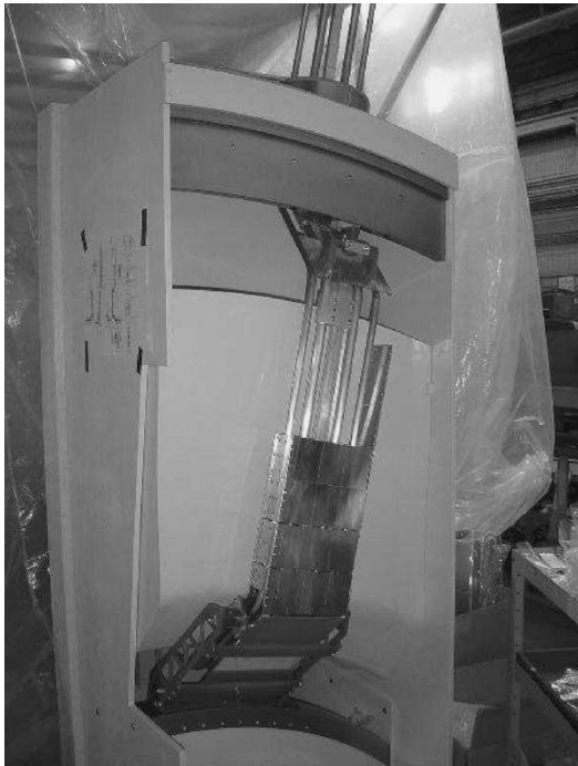
Fig. 3. Mock-up of the cryostat bulkhead and feedthrough.
