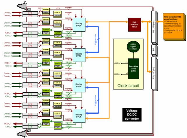
Figure 7: 9U Optical Multiplexer Board.
