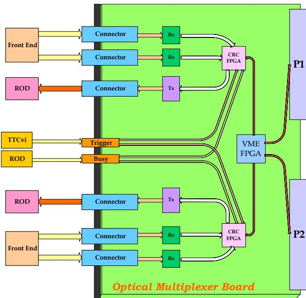
Figure 2: Optical Multiplexer Board Block Diagram.
