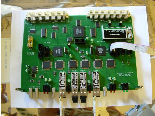
Figure 6: Optical Multiplexer Board.
