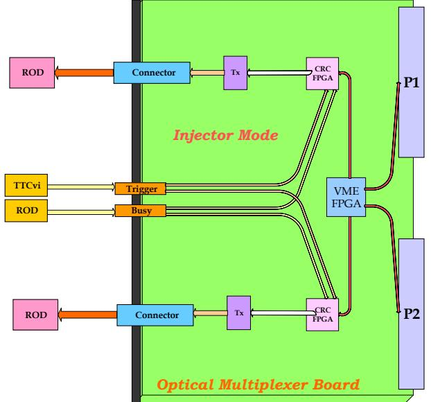
Figure 4: Data Distribution in Injector Mode.
