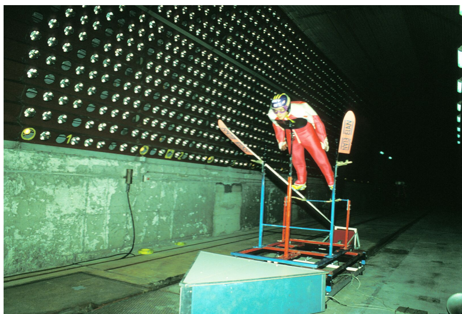
Fig. 4: Wind tunnel measurements: The aerodynamic forces largely depend on the flight style. Large-scale wind tunnel in Vienna; Andreas Goldberger, wr 225 m (2000).
