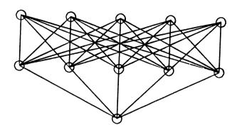
Fig. 1: Schematic view of a normal layered feed-forward network with one hidden layer (the neurons are represented by circles and the connections by lines).
