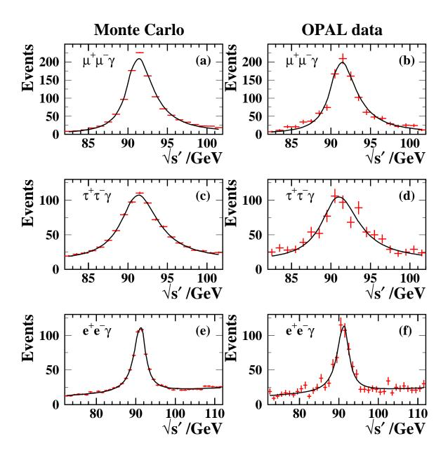
Figure 4: Fits of Eq. (1) to Monte Carlo (left-hand plots), combining samples generated at energies in the range 183–209 GeV, and OPAL data (right-hand plots) collected in the years 1997–2000 at the same nominal energies, for muon-, tau- and electron-pair events respectively. The Monte Carlo expectation is normalised to the integrated luminosity of the data in each case.
