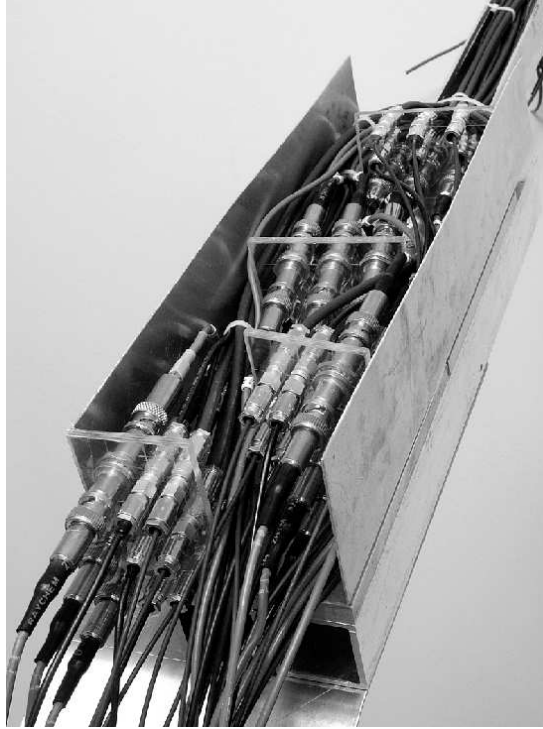
Figure 2.14: T0 patch panels inside the duct on the top of the muon absorber.
