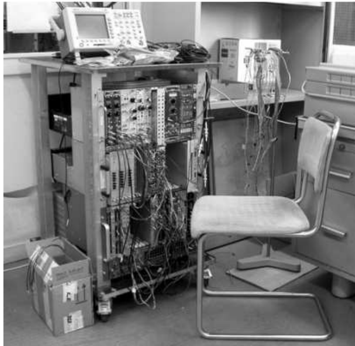
Figure 2.44: Test version of the main T0 electronics rack photographed during the 2004 run at CERN.
