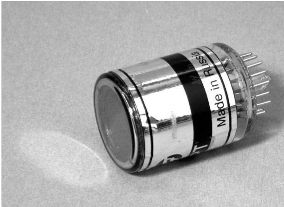
Figure 2.2: FEU-187. The outside diameter of the photomultiplier tube is 30 mm.
