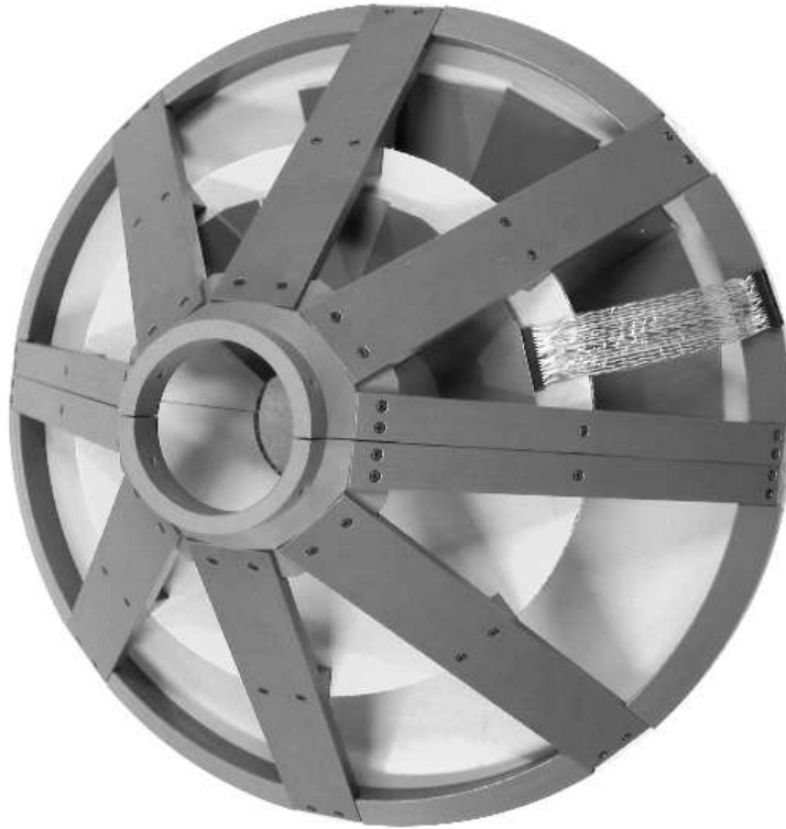
Figure 4.20: Photograph of model showing the assembly of the FMD3 inner and outer silicon ring (partly equipped in upper half) inside its support cone. The cone and the detector support plates can be split along the horizontal axis.
