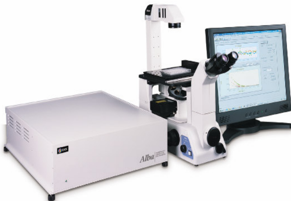
Fig. 3.4.1. The FCS Alba™ Microspectrometer System manufactured by ISS Co., (Urbana, Illinois, USA). The inverted, epi-fluorescence microscope shown in the figure is the Nikon TE-300 –special Model, that has available both a back illumination port and a left-hand side port. The PC employed for data acquisition, storage and processing is located behind the instrument, as is the laser illumination source (not visible in the figure).
