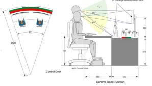
Figure 2: Proposition of CCD for the layout of the generic console in the CCC.
