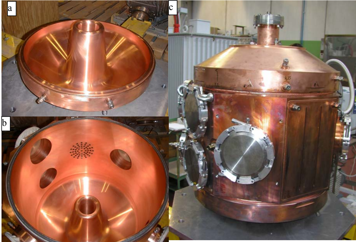
Fig. 1: a) The end-cap with the nose cone; b) the central part on the nose cone, c) the three pieces assembled vertically in order to perform the measurements.
