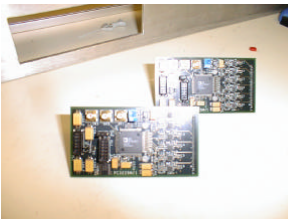
Figure 5: The cross-point switch based electrical test cards.
