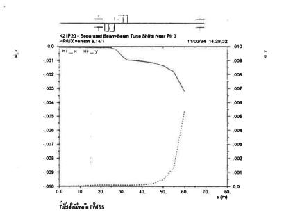
Figure 11: Beam-beam tune shifts  $\xi_x$  and  $\xi_y$  near Pit 3 in the standard K21P20 configuration. The electrostatic separators ZL are excited.
