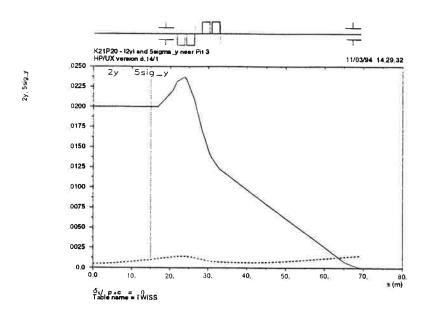
Figure 7: Vertical orbit separation 2|y| and beam size  $5\sigma_y$  near Pit 3 in the standard K21P20 configuration. The electrostatic separators ZL are excited.
