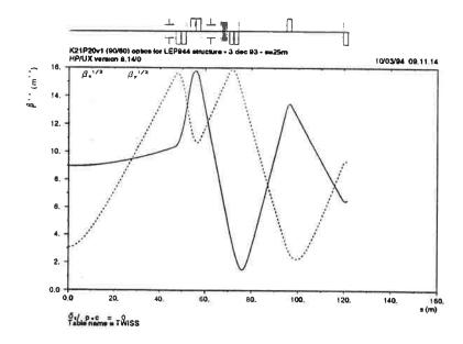
Figure 4: Orbit functions  $\sqrt{\beta_x}$  and  $\sqrt{\beta_y}$  near Pit 1 in the modified K21P20 configuration.
