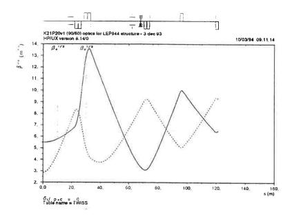
Figure 3: Orbit functions  $\sqrt{\beta_x}$  and  $\sqrt{\beta_y}$  near Pit 1 in the standard K21P20 configuration.
