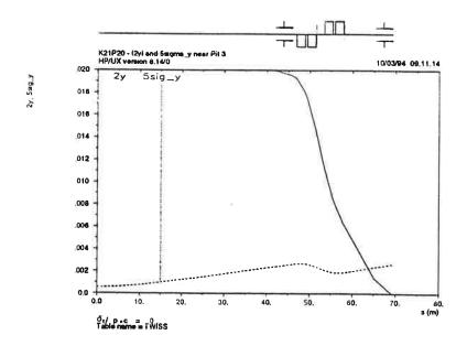
Figure 8: Vertical orbit separation 2|y| and beam size  $5\sigma_y$  near Pit 3 in the modified K21P20 configuration. The electrostatic separators ZL are excited.
