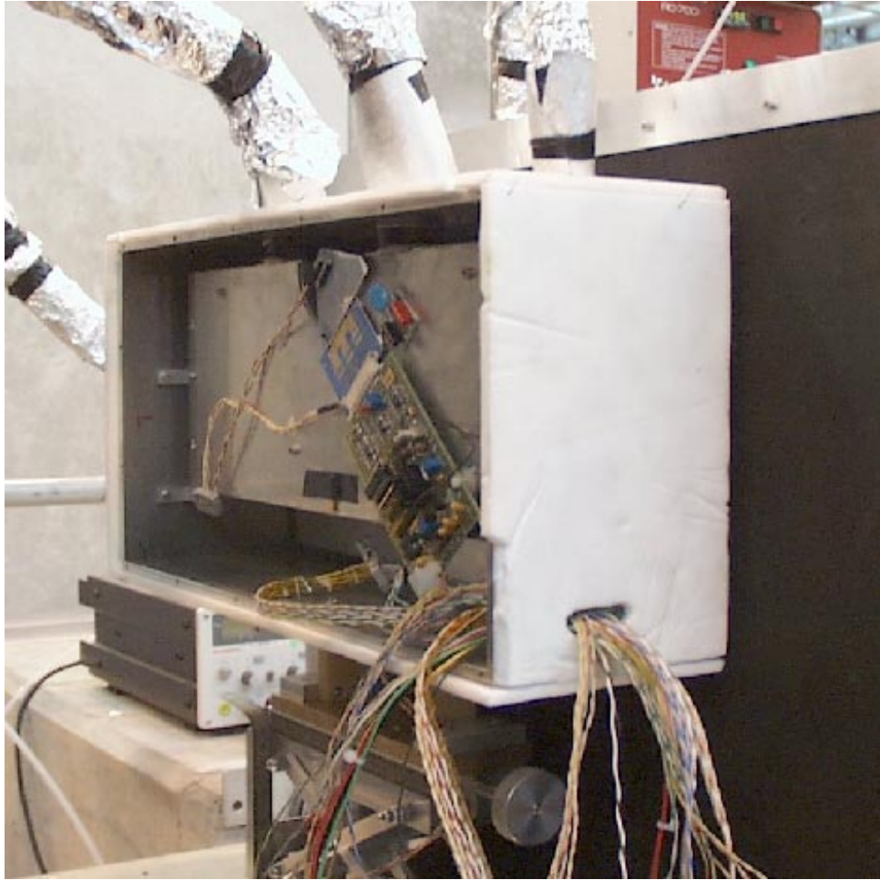
Figure 5: The irradiated test detector in its insulating box. The box containing the second telescope station is visible behind the insulating box. The fridge is visible in the top right of the photograph along with the pipes connecting this to the test detector.
