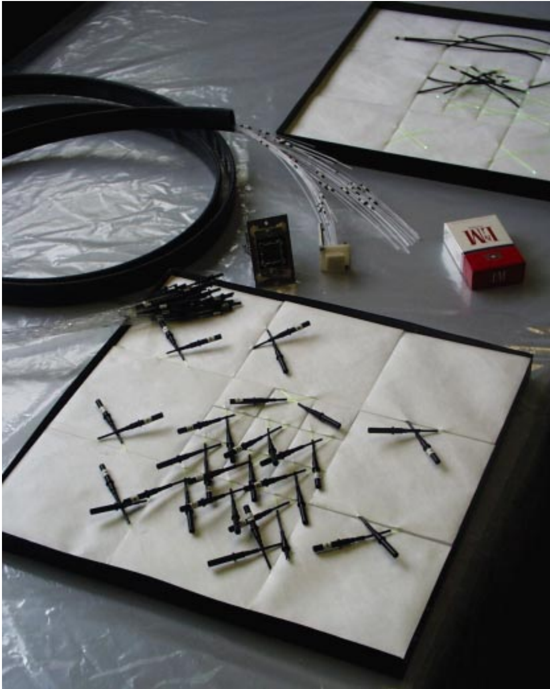
Figure 9: Common view of assembled prototypes. Ends of WLS fibres are equipped with optical connectors. Bundle of clear cables is inserted in light isolating tube. 3m clear fibres go to special optical connector which provides precise positioning fibres to corresponding PMT anode pixels.
