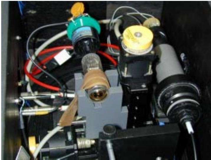
Figure 2-6 View of the PMT under test fixed on the moving table and the reference PMT on the left
