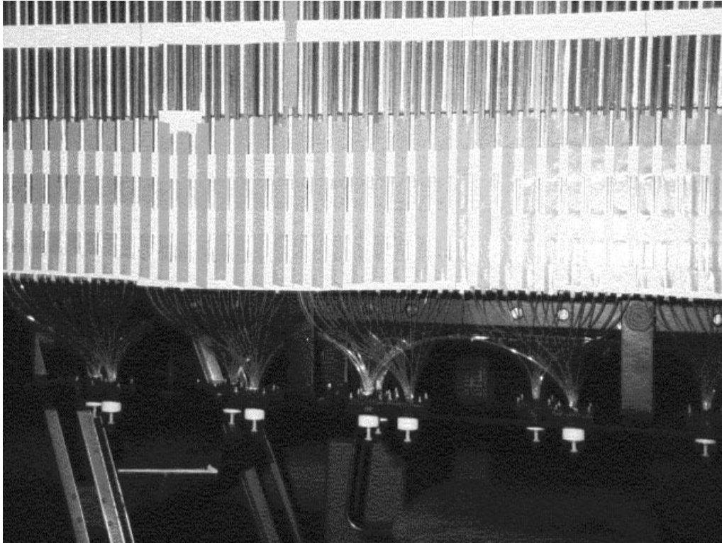
Figure 5: The module outlook after optics assembly. White cup's on the bottom contain glued fiber end's.
