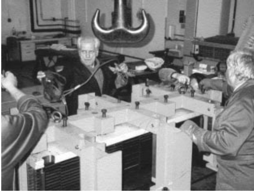
Figure 3: The submodule assembly tool. Stack of glued plates are being pressed by thick cover.
