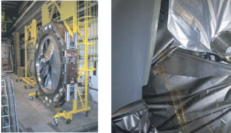
Figure 12: Large drift chamber after the implosion of the vacuum chamber. Courtesy of NA 48.
