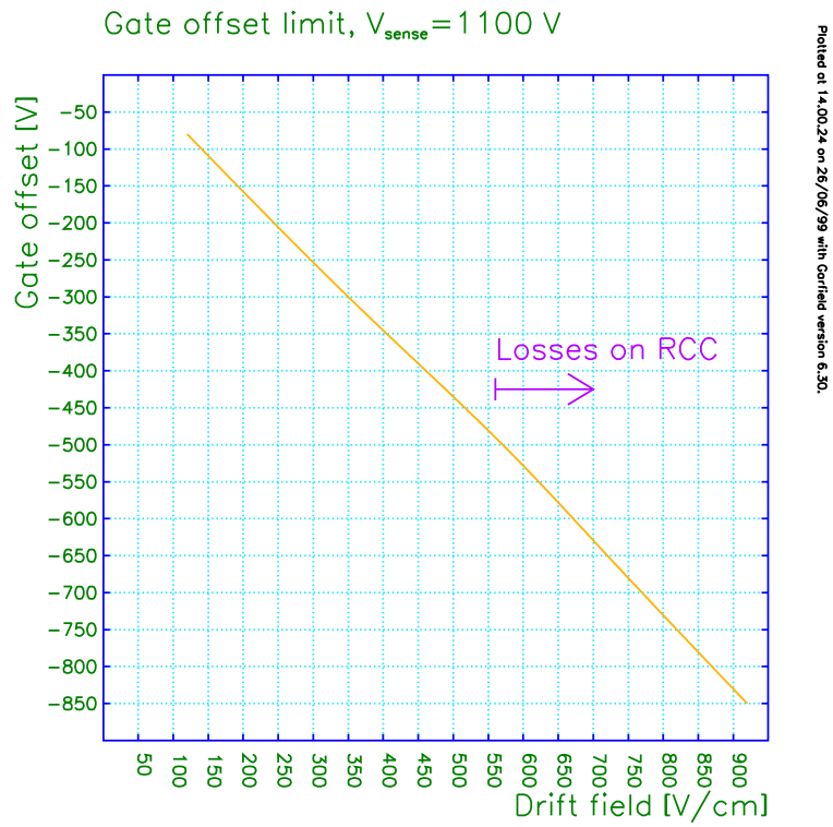
Figure 73: Dependence of gate voltage on drift field for a given sense wire voltage setting of 1100 V. The arrow indicates the regions where electrons are starting to be lost
