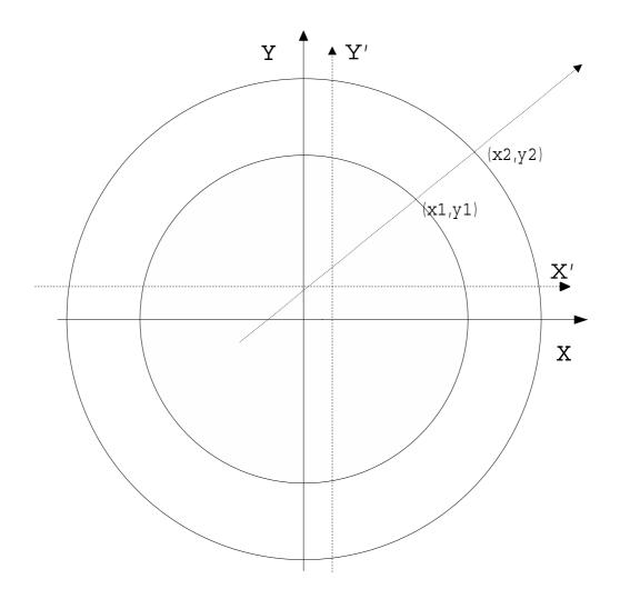
Figure 5: Geometrical sketch of the two  $\mathfrak{P}$  ixel layers with the reconstructed points in the transverse plane. Correlation between the points  $(x_1, y_1)$  and  $(x_2, y_2)$  may be used to determine the distribution of the intercepts with axes X', Y' (estimated from a first-order evaluation of the vertex coordinate).
