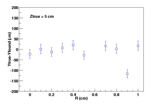
Figure 8: Difference between  $y_{true}$  and  $y_{found}$  as a function of the radial distance of the vertex location from the z-axis.
