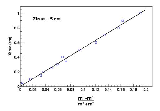
Figure 3: Correlation between the true x-position of the vertex and the asymmetry parameter originating from the left and right multiplicities of the reconstructed points in the first pixel layer.
