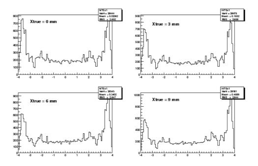
Figure 2: Multiplicity of reconstructed points in the first pixel layer, projected along x, for several values of the nominal vertex position  $x_{true}$ . Central PbPb collisions, with a particle density  $(dN_{ch}/d\eta)_{\eta=0}=8000$ .
