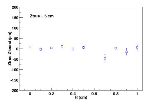
Figure 9: Difference between  $z_{true}$  and  $z_{found}$  as a function of the radial distance of the vertex location from the z-axis.
