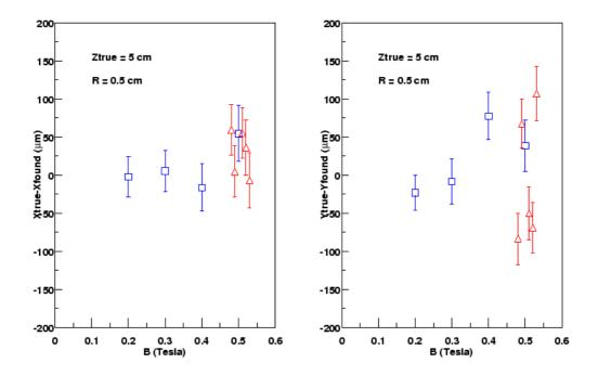
Figure 14: Differences  $x_{true}$ - $x_{found}$ ,  $y_{true}$ - $y_{found}$  as a function of B, for a radial distance R=5 mm. The last 6 points on the right refer to events at the same magnetic field (B= 0.5 T), which are only plotted slightly shifted to show statistical fluctuations.
