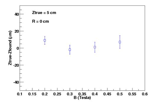
Figure 12: Difference between  $z_{true}$  and  $z_{found}$  as a function of the magnetic field setting.
