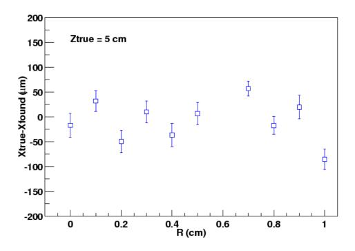
Figure 7: Difference between  $x_{true}$  and  $x_{found}$  as a function of the radial distance of the vertex location from the z-axis.
