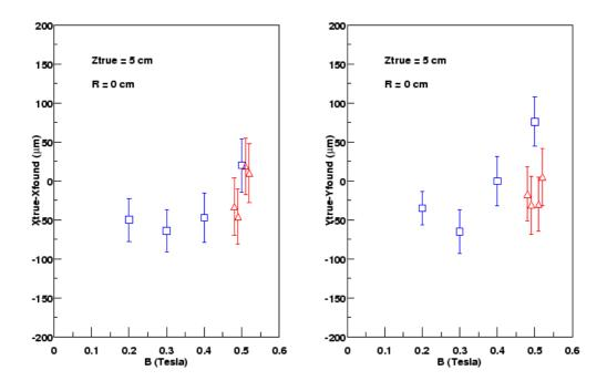
Figure 13: Differences  $x_{true}$ - $x_{found}$  and  $y_{true}$ - $y_{found}$  as a function of B, for a radial distance R=0. The last 5 points on the right refer to events at the same magnetic field (B= 0.5 T), which are only plotted slightly shifted to show statistical fluctuations.
