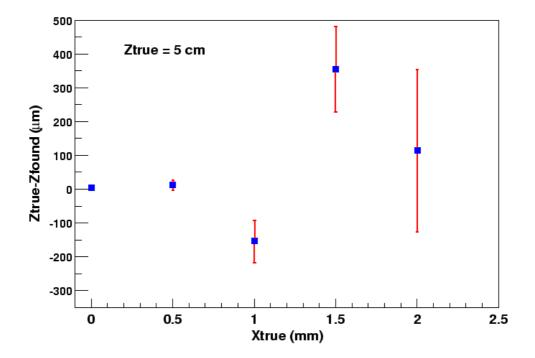
Figure 1: Difference between  $z_{true}$  and  $z_{found}$  and vertex resolution (reported as error bar on each point) for vertex locations away from the z-axis. In this case no correction has been introduced for the x and y-position of the vertex. PbPb central collisions, with a particle density  $(dN_{ch}/d\eta)_{\eta=0}=8000$ .
