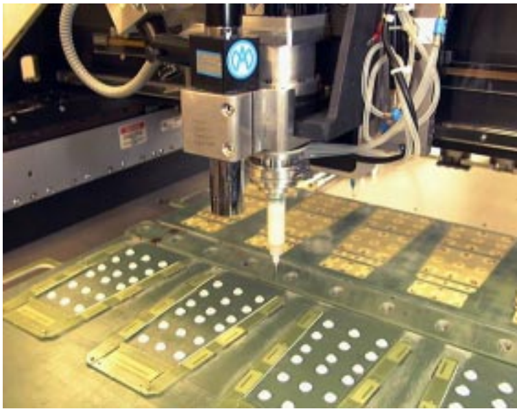
Figure 17: Photo of glue dispenser tool in action.
