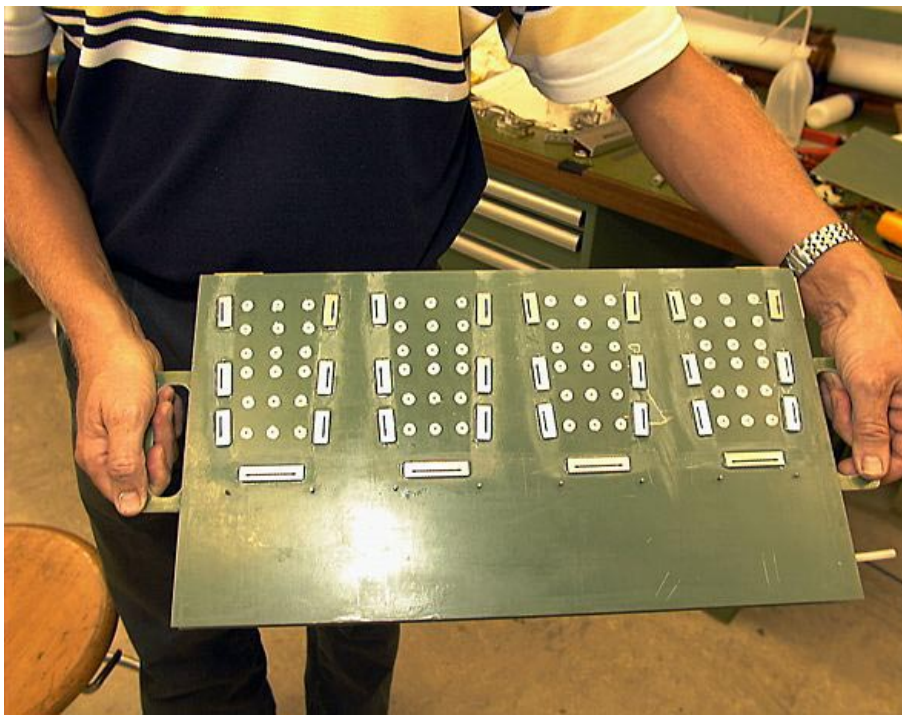
Figure 11: Photo showing the top face of the assembly platform. The small white circles are the teflon vacuum chuck contact pads for the sensors and the rectangles are the aluminium vacuum chuck contact pads for the CF-frames.
