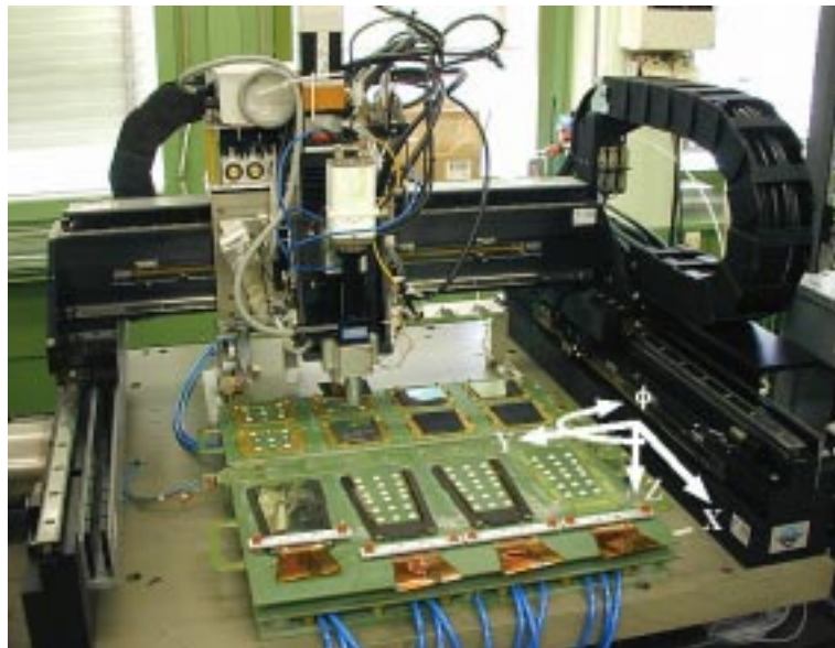
Figure 4: Closeup view of the gantry setup showing the assembly and sensor platform in the front and the vacuum tool rack in the back. The coordinate system used in the gantry setup is shown in the bottom right corner.
