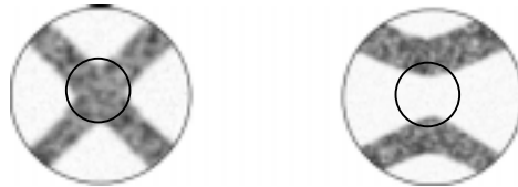
Figure 2. Interference picture on the output of the electro optical shutter: zero applied voltage (shutter closed) – left, half-wave voltage (shutter opened) – right. The input of the shutter is limited to 4mm by the input diaphragm (outer ring). The spatial zone of the maximum beam intensity is marked with the inner ring.
