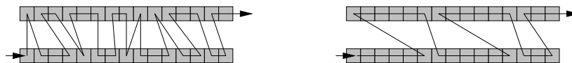
Figure 7: A logical access pattern to two collections (left) and the physical pattern after read-ahead optimisation (right)
