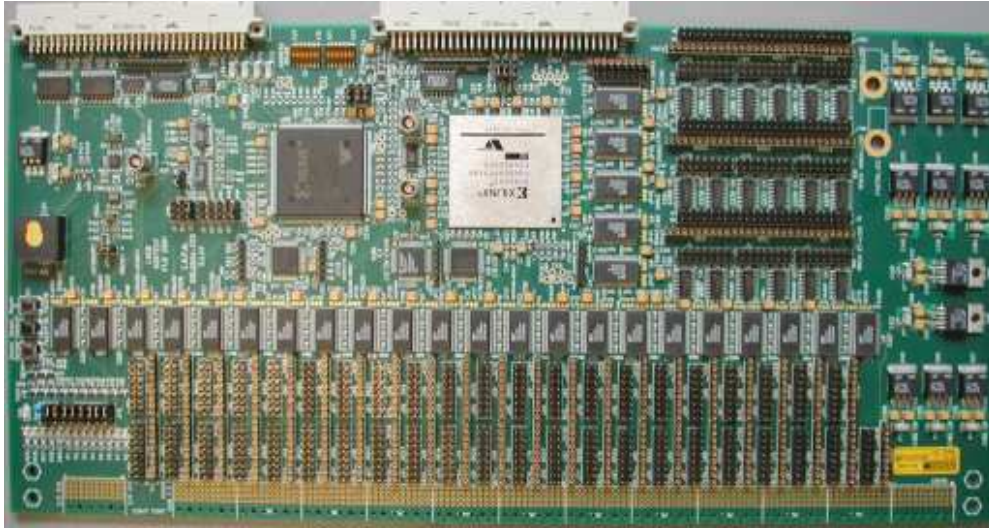
Figure 4: The Processing Unit test board. The Processing Unit has been implemented in a single FPGA. The board allows to test the cluster selection algorithm on 8 input channels.
