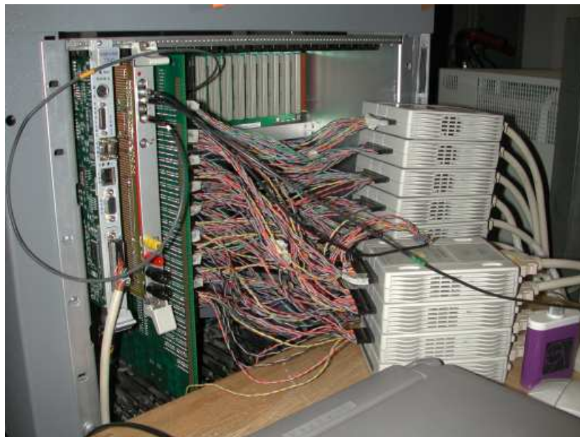
Figure 5: The setup arranged to test the Processing Unit prototype. The board is fed by a Pattern Generator which allows injecting 32-bits pattern (pseudo-clusters) at 40 MHz. Data outputs have been recorded by a Logic Analyzer and then compared to the expected ones.
