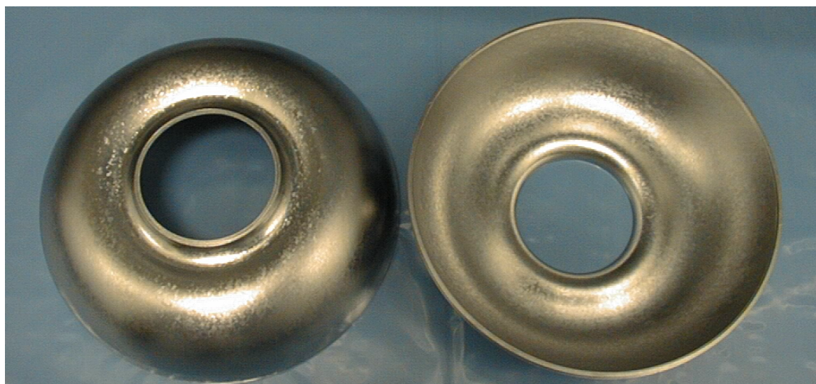
Fig. 4. 1300 MHz reentrant cavity cups. Left cup: outside surface view, right cup: inside surface view.
